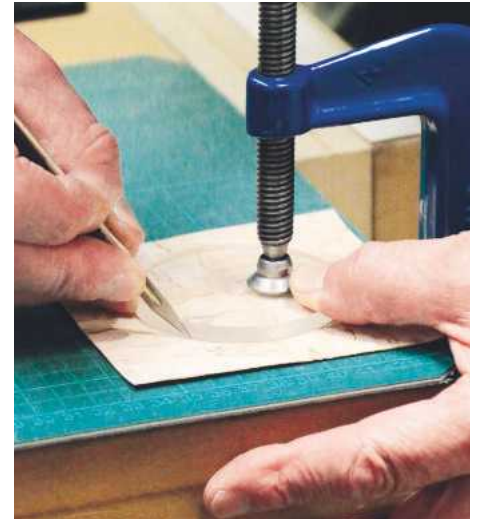
Using a template, a scalpel cuts the centre circle
